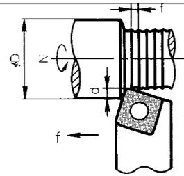
N : Work Rotating speed (rpm)
