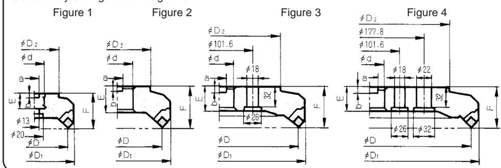
( D : External Diameter,  $D_1$  : External Diameter of Body,  $D_2$  : External Diameter of Boss, d : Hole Diameter, F : Height, E : Thickness, a : Width of Key Way, b : Depth of Key Way)
