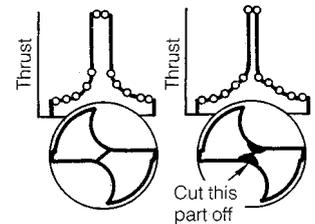
The thinning makes concentrating thrust small. This means easy cutting, good chip removal and longer tool life.
