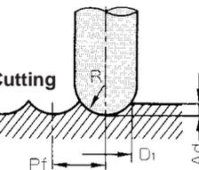
**- Calculation of Speeds and Feedrate for the Ballnose endmills are the same as those for Normal endmills**
